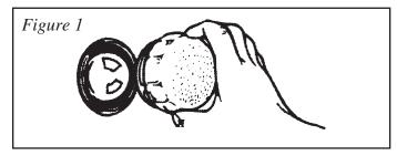
3. Replace bulb with a 40 watt appliance bulb, available at any hardware store.
