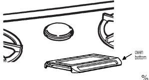
Hot air and moisture escape from the oven through a vent in the center rear of the cooktop. **Do not block the vent.** Poor baking/roasting and bad combustion can result.
