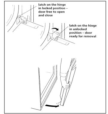
Completely open oven door. In both back corners of the door you will see door latches in the locked position. Rotate both latches forward to the unlocked position.
