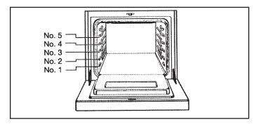
Your oven has five rack positions. Rack position 1 is the lowest position, or closest to the bottom of the oven. Rack position 5 is the highest position, or farthest from the bottom of the oven.
