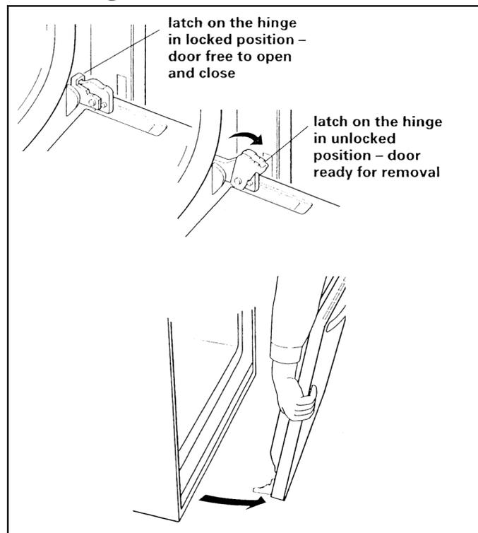
Completely open oven door. In both back corners of the door you will see door latches in the locked position. Rotate both latches forward to the unlocked position.
