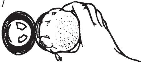
3. Replace bulb with a 40 watt appliance bulb, available at any hardware store.
