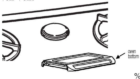
Hot air and moisture escape from the oven through a vent in the center rear of the cooktop. **Do not block the vent.** Poor baking/roasting and bad combustion can result.
