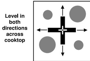
The range must be level in order to assure uniform cooking and baking. Shim legs if required.
