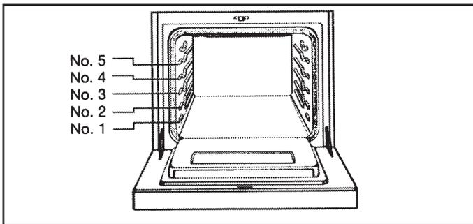
Your oven has five rack positions. Rack position 1 is the lowest position, or closest to the bottom of the oven. Rack position 5 is the highest position, or farthest from the bottom of the oven.
